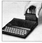
16K MEMORY MODULE: Like any powerful, full fledged computer, the ZX81 is expandable. Sinclair's 16K memory module plugs right onto the back of your ZX81 (or ZX80, with or without 8K BASIC). Cost is \$99.95, plus shipping and handling.
